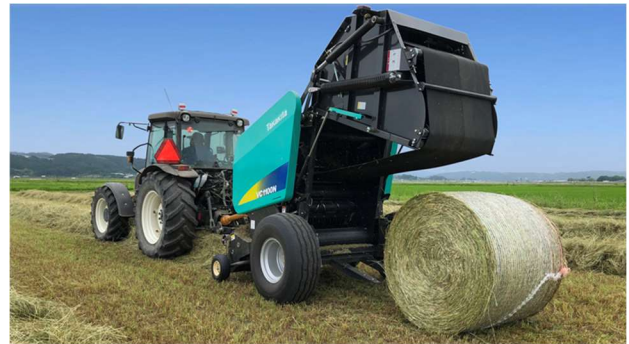
An example of TAKAKITA's products. Variable Diameter Round Baler; Bale Size:φ70-115cm.
