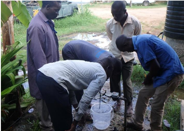
Meter accuracy testing by using a scaled bucket
