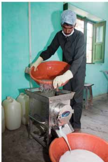
Extracted gel goes through a five process filtration
