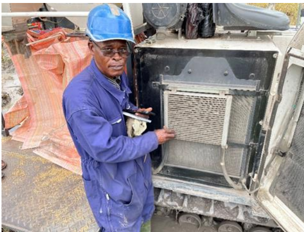
M. Kanga, the SIMAPRESS operator, showed us where to inspect and clean during maintenance.
