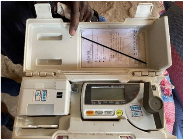
PRORIL2, another JICA project, donated Kett moisture testers to some millers in Yamoussoukro and surrounding Districts, One such miller in Bouaké showed AFICAT Team the tester, Riceter f501, which he usually uses when he purchases paddy from farmers to maintain fair trade.
