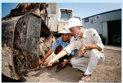
Mr. Tsunabuchi Masaki is checking the condition of heavy equipment and its parts with CMAC Staff in CMAC Central Workshop in Battambang. Equipment for demining activities is damaged by blasting operation. If the maintenance of equipment is not appropriate, a life of operator will be in danger and repair cost will be higher than maintenance cost.
