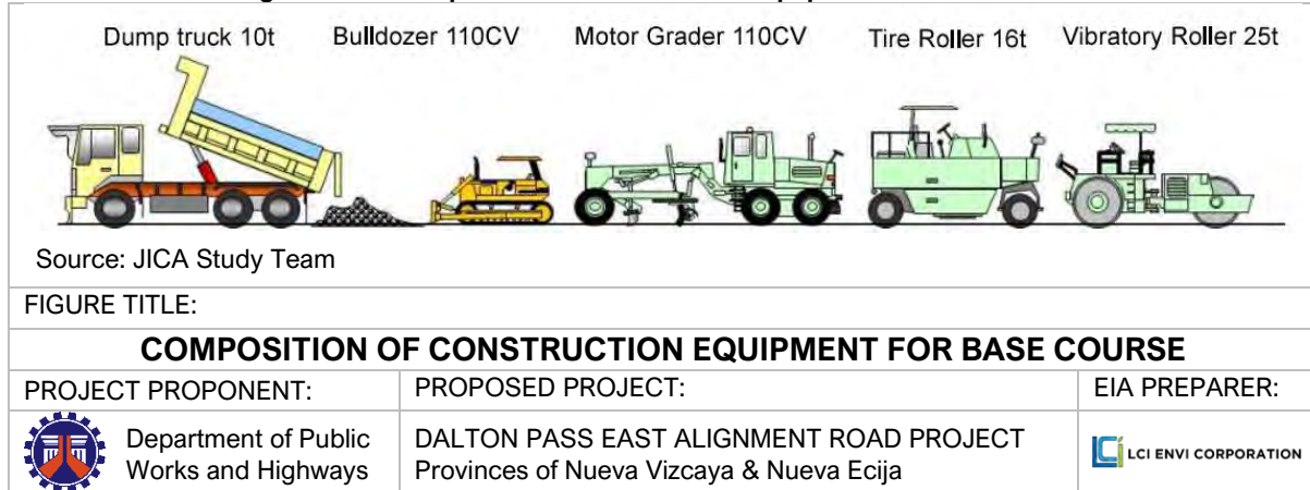
Figure 1-22: Composition of Construction Equipment for Base Course
