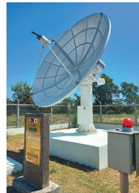
Philippines: An antenna for a local user terminal (a ground satellite data receiving station) provided under the Project for Development of Extreme Weather Monitoring and Information Sharing System. With the use of satellite data thus received, the project developed a system to forecast extreme weather events.
