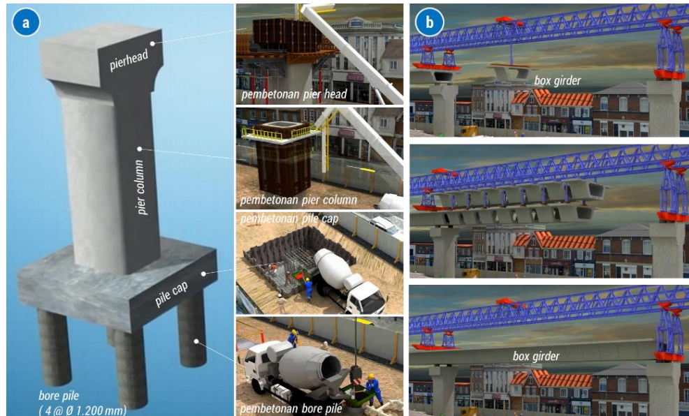
Figure 2.24. Illustration of Elevated Station Support Pole Construction
