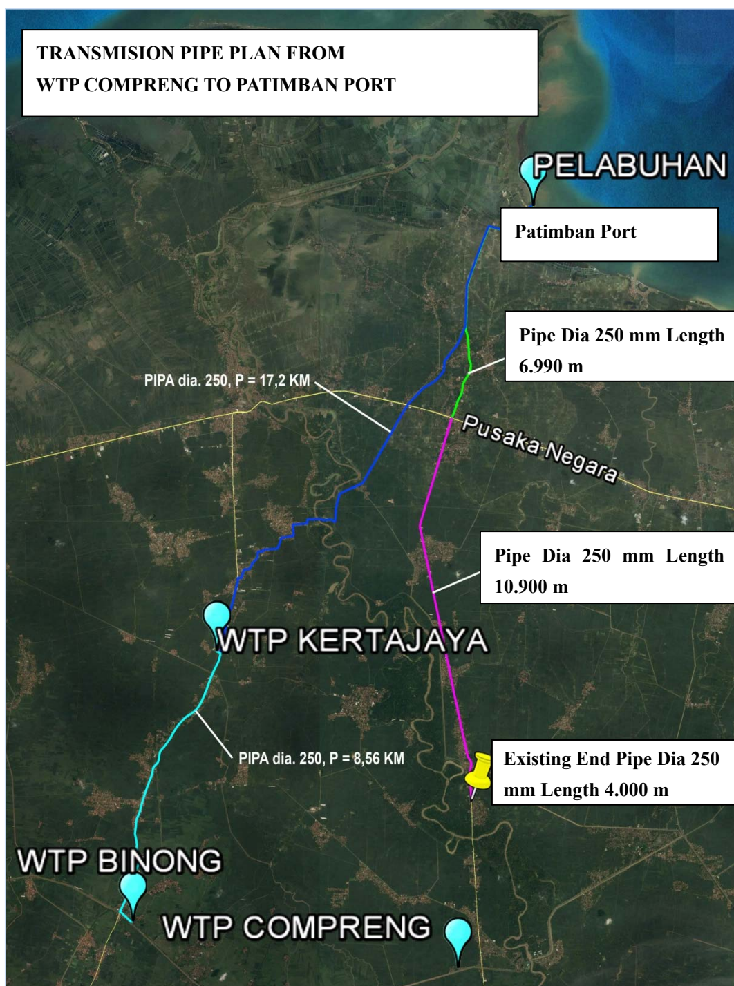
Figure 3.3-3 Transmission Water pipe line from Water Treatment Plant at Compreng to Patimban Port
