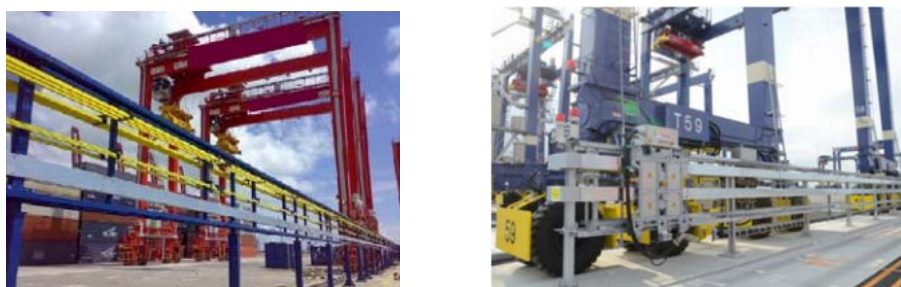
Figure 3.3-58 Power supply by trolley cable
