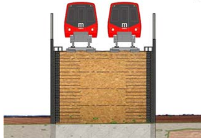
Figure 1.4.2 Cross-section of typical Embankment
