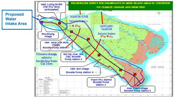
Figure 2.3.26 Extension Plan of Intake and Pipeline for Rural Water Supply in South Ben Tre Source: Center of Rural Water and Environment Sanitation Ben Tre Province
