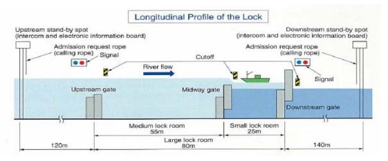
Figure 2.3.30 Example of Lock to Prevent Saltwater Intrusion
