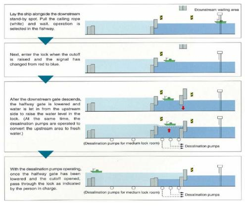
Figure 2.3.31 An Example of Lock Operation to Prevent Saltwater Intrusion Source: Information of Nagaragawa Estuary Barrage, Japan Water Agency
