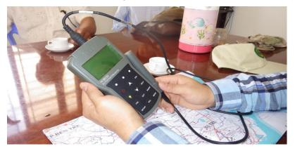
Figure 2.3.12 Salinity Concentration Meter used at Son Doc 2 Sluice Source : JICA survey team (2016)
