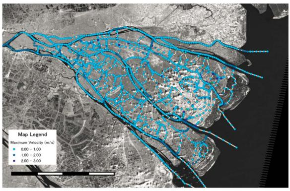
Figure 2.3.8 Distribution of Maximum Velocity (Calculated with Existing Condition) Source : JICA survey team (2016)
