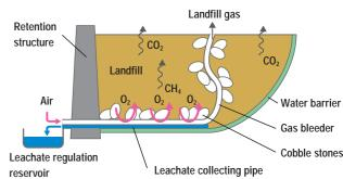
Structure of the Fukuoka Method (semi-aerobic landfill system)
