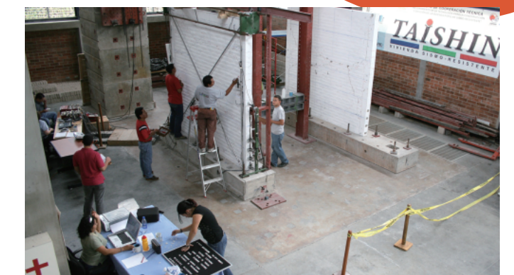
A model house under construction displaying new earthquake-resistant building techniques (upper left). A wall is tested to determine its ability to withstand an earthquake.
