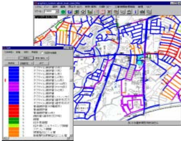
Fig. 13 Classification of pipe material
