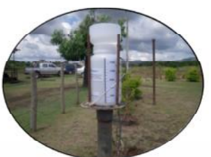
Type of rain gauges that are used for community Flood early warning
