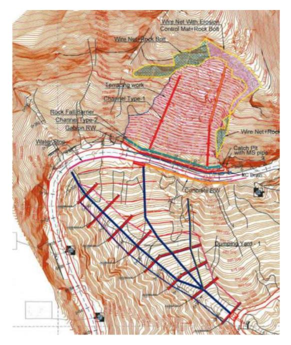
Total devastated hillside area for the site is 11 Ha with maximum slope gradient of 60 degree. Out of which, 2 Ha will be treated where hillside work such as cut slope work, wire netting with rock bolting, retaining wall work, mat work, channel work, fence works are planned.
