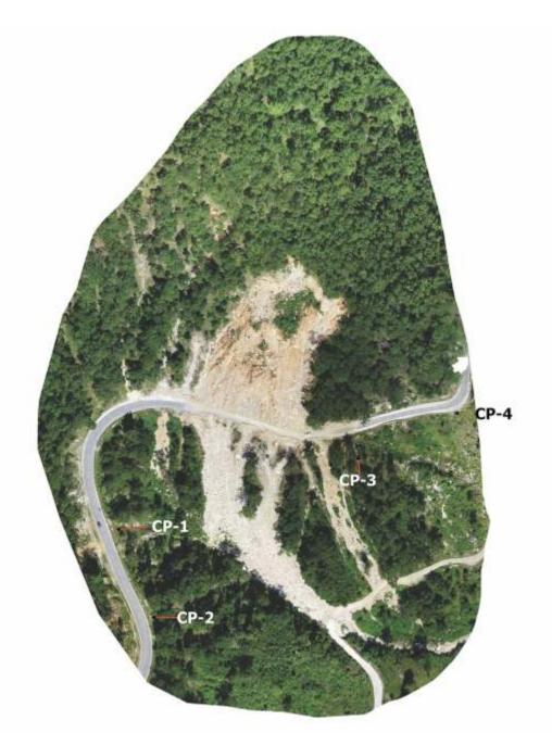
This is a slope failure type disaster site. The site locates near northwest border of Uttarakhand about 60 kms from Pithoragarh city on Delhi - Dhaarchulha Highway. A huge soil mass at the top of the slope failed and has become very vulnerable. Rocks and loose debris had erupted after the slope failure was affected by the subsurface water. The current primary cause of sediment runoff is erosion by surface water during rainfall.
