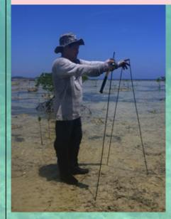
Sediment depth determination using steel rod
