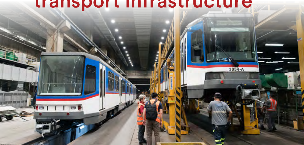
Refurbishment of MRT-3 cars
