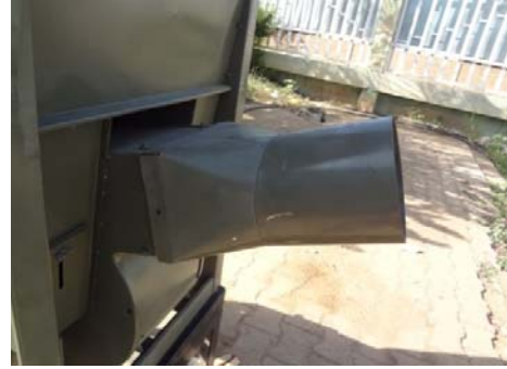
Husk blower & duct
