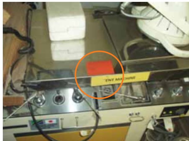
Red tag place on unnecessary equipment
