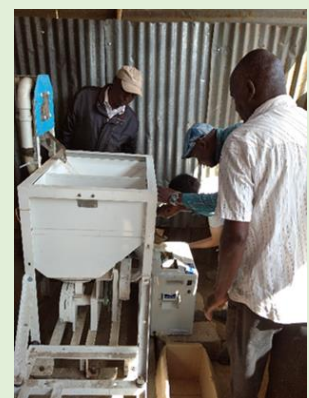
A small-scale miller is processing rice using a Kanryu rice mill equipped with a destoner.
