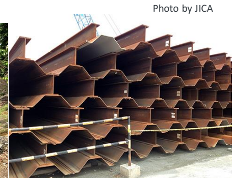
(Left photo) Marimango drainage channel to be repaired (Right photo) Hat-shaped steel sheet piles and H - shaped steel to be used in the project (Japanese technology)
