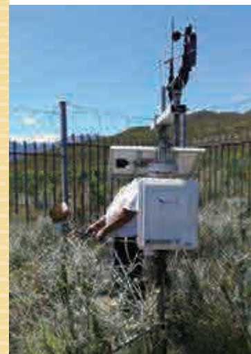
One of the six automatic weather stations for seasonal change forecasting installed under this SATREPS project
