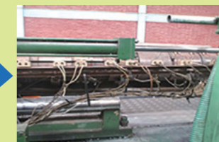
After Kaizen. The machine has stopped leaking oil and the wires are well-organized.
