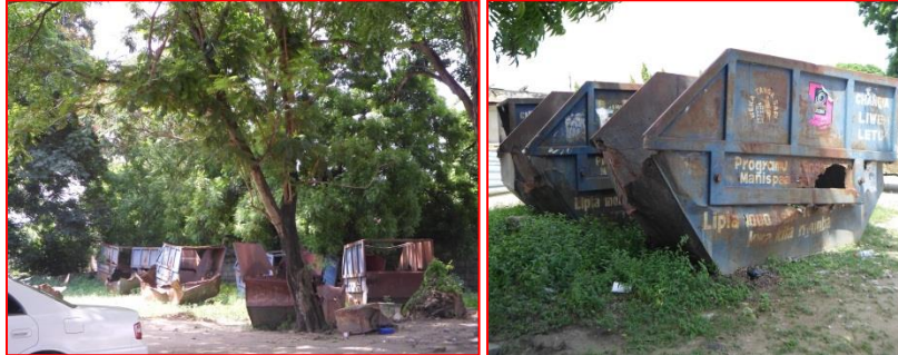
Rotting skipbuckets due to humid weather
