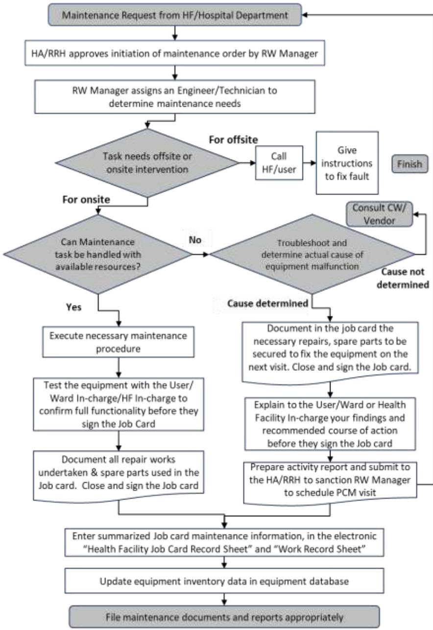
Fig 4: RW Maintenance Work Flow Chart
