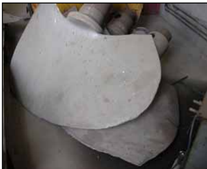
Figure 5: Turbine damaged by quartz silt
