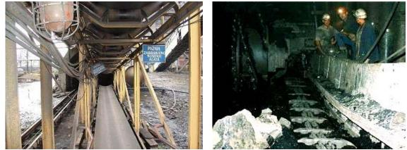
Conveyor installed in main tunnel and underground coal excavation and transportation system (Breza Coal Mines)
