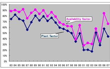
Figure-3 Trend of plant load (capacity factor) and availability factor of facilities
