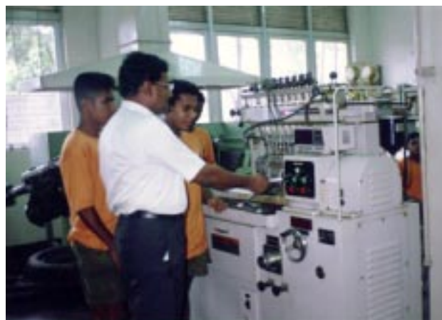
Trainees being instructed in the use of testing devices for diesel engines
