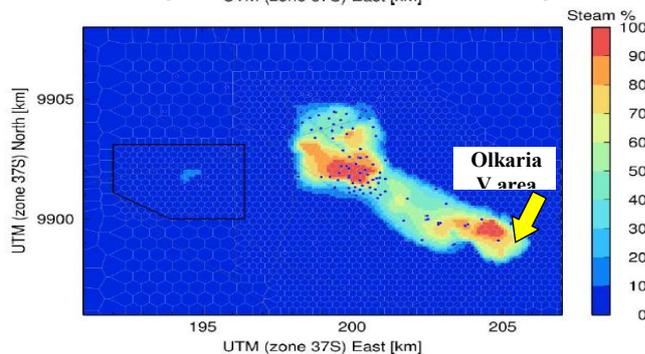
**Figure 55.** Steam fraction in the main production layers, E (top, EPF), H (centre, NEPF) and J (bottom, Domes) at the end of the forecasting period for Scenario 6 with injection.
