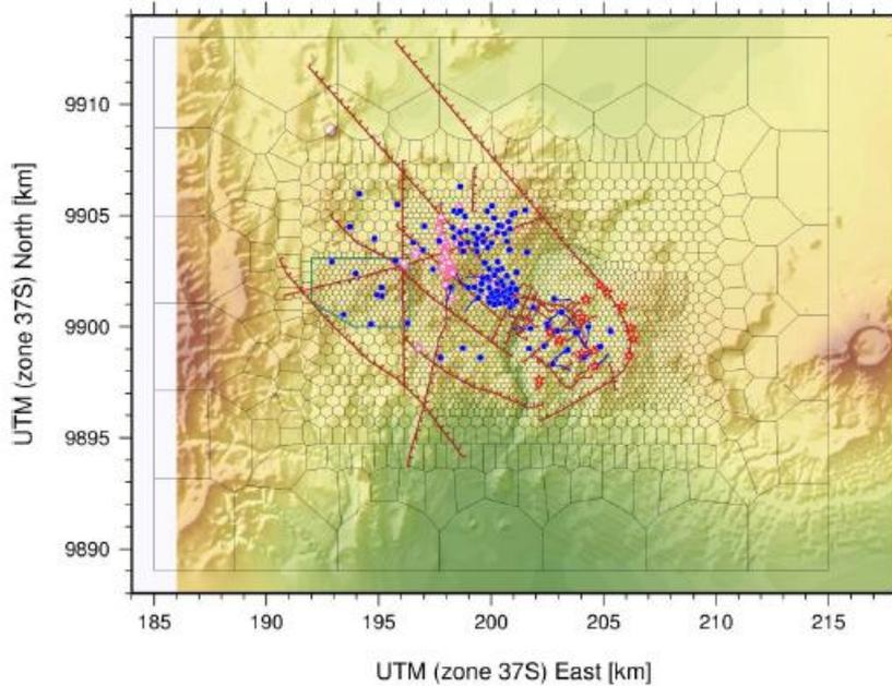
**Figure 17.** Plan view of the model grid and main structures in the Greater Olkaria geothermal system. Well locations are shown with blue dots, surface manifestations with pink triangles and rhyolite eruption centres with red stars.
