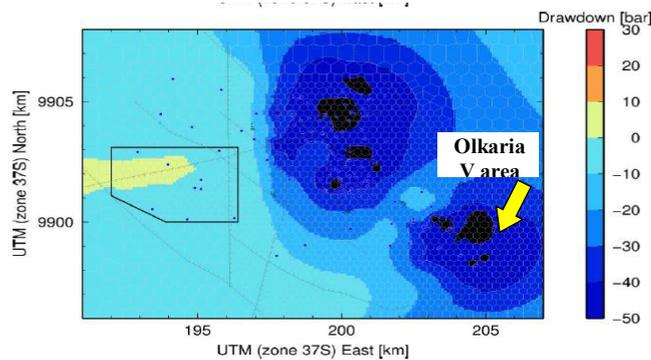
**Figure 54.** Drawdown in the main production layers (E top, H centre, J bottom) at the end of the forecasting period for Scenario 6 with injection.
