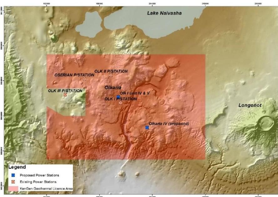
**Figure 2.** Map of the Greater Olkaria Geothermal Area showing KenGen’s concessions area and the location of present power plants and the planned expansion of Olkaria I and the new Olkaria IV.
