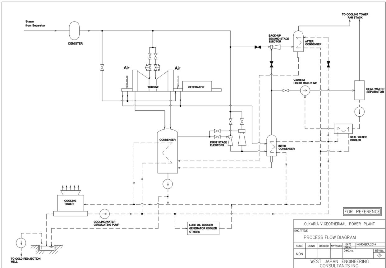
Fig. 3.3.1-5 Plant Process Flow Diagram (Preliminary)
