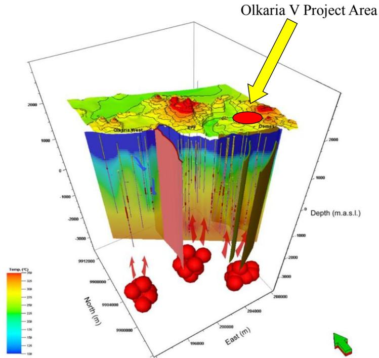
**Figure 4.** A schematic sketch of the present revision of the conceptual model of the Greater Olkaria Geothermal System. The green arrow in the bottom right corner is directed north. The top layer shows the topography and the Ololbutot fault is shown along with parts of the ring structure. A temperature cross section is also shown and at the bottom the postulated heat sources and up-flow zones (Mannvit/ISOR/Vatnaskil/Verkis, 2011c).
