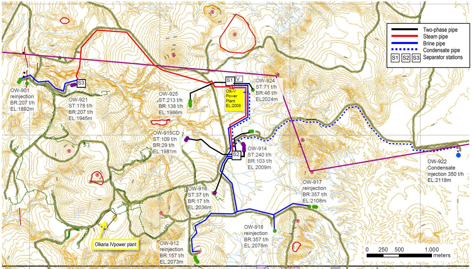
Fig. 3.3.1-1 Proposed location of Olkaria V power plant and steamfield layout
