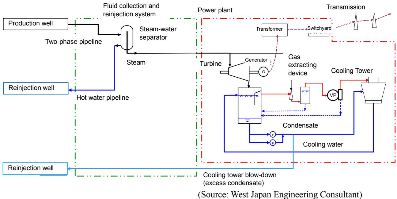
Fig.1.2-2 Overview of fluid collection and reinjection system
