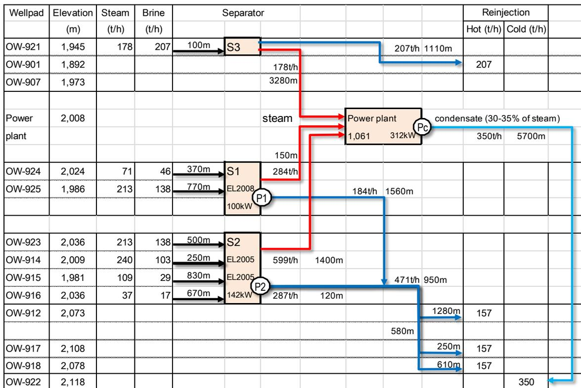
Fig. 3.3.3-1 Configuration of Steamfield
