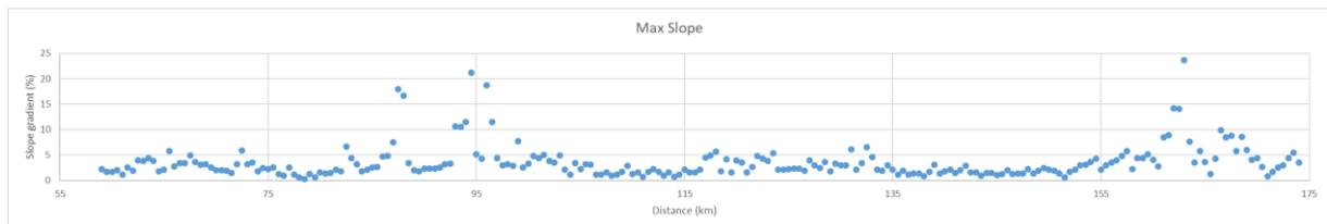
**Figure 6-20** Maximum slope perpendicular to road alignment from 59.0 km to end of the route (measured at 500 m intervals over distance 200 m either side of the alignment)
