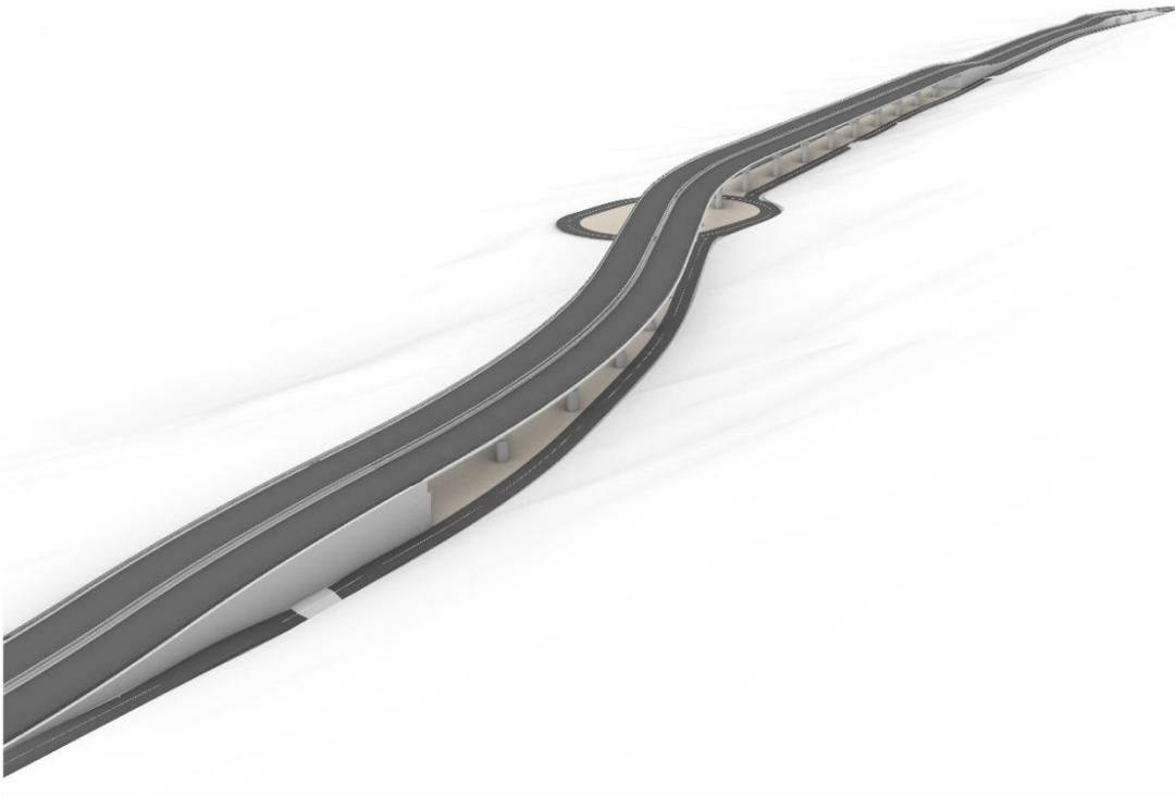
**Figure 4-8** 3D Representation of the Second Flyover Section over Nakuru's 2<sup>nd</sup> Roundabout with a View on the Embanked Section
