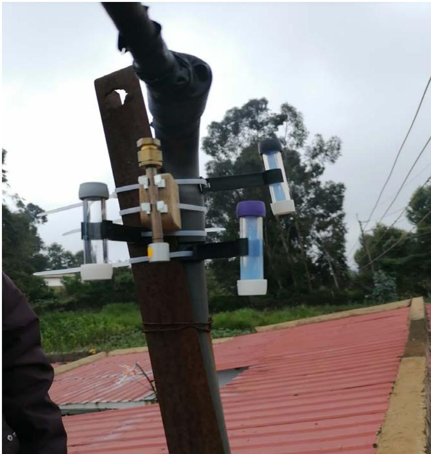
Passive Air samplers at sampling point A1
