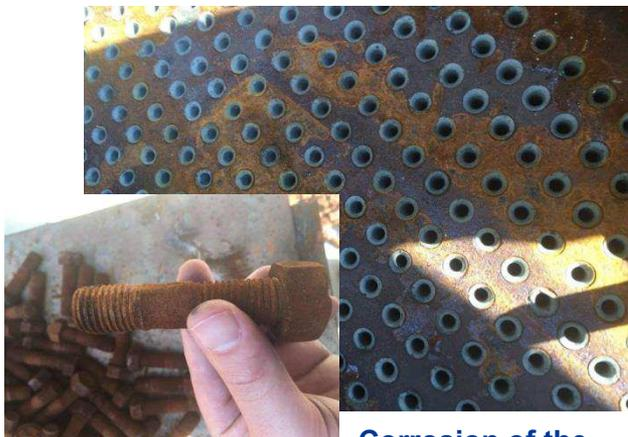
Corrosion of carbon steel bolt.
