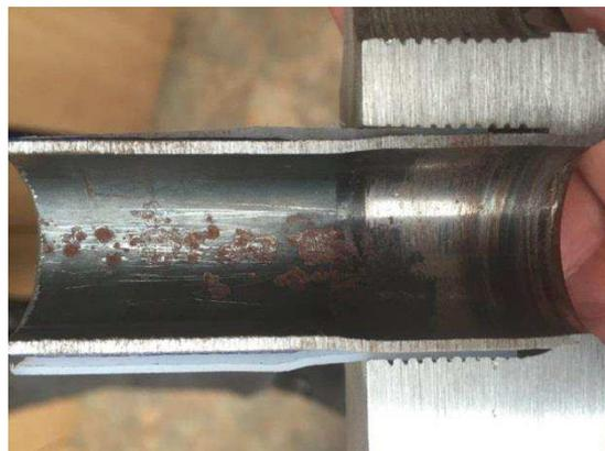
Corrosion of a carbon steel tube.
