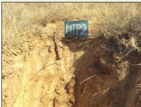
*Figure 3: Typical test pit investigated on site (shallow refusal)*
