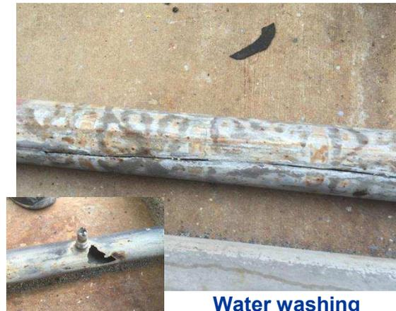
Wear damage of carbon steel tube.
