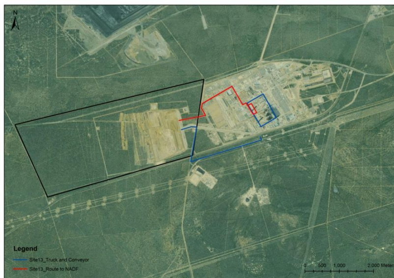
Figure 4.7: Proposed transport routes to site 13 (NADF – Northern Ash Disposal Facility)
