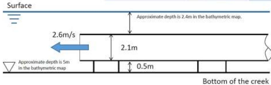
**Figure 6-10 Outfall Configuration for 300MW Case**
