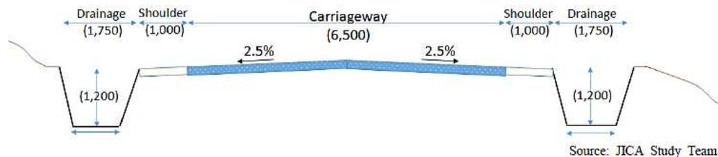
*Figure 2-18 Planned Standard Road Cross-section*
