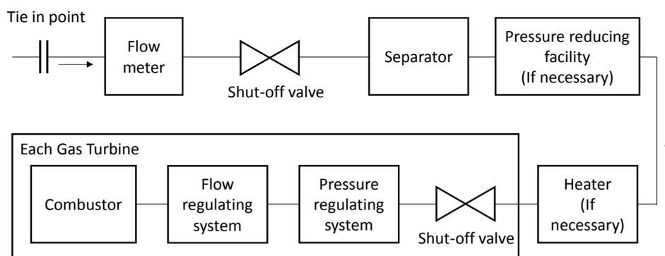
**Figure 2-32 Preliminary Flow Diagram of Gas Supply System**
