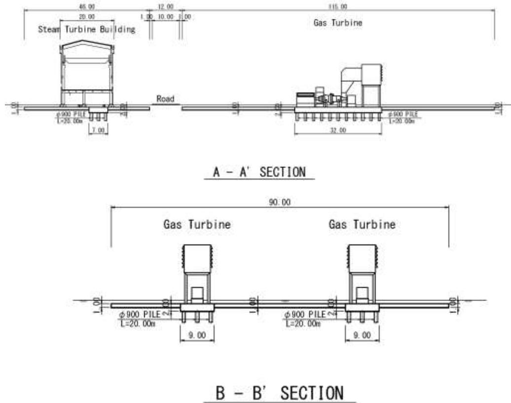
**Figure 2-27 Draft Design of Foundation for GT and ST**
