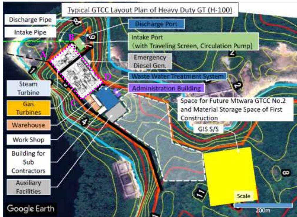
**Figure 2-5 Layout of Project Components**
