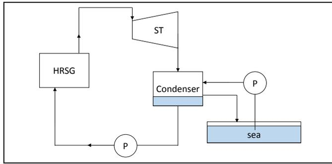
**Figure 2-9 Schematic System Diagrams of ST Cooling Type**
