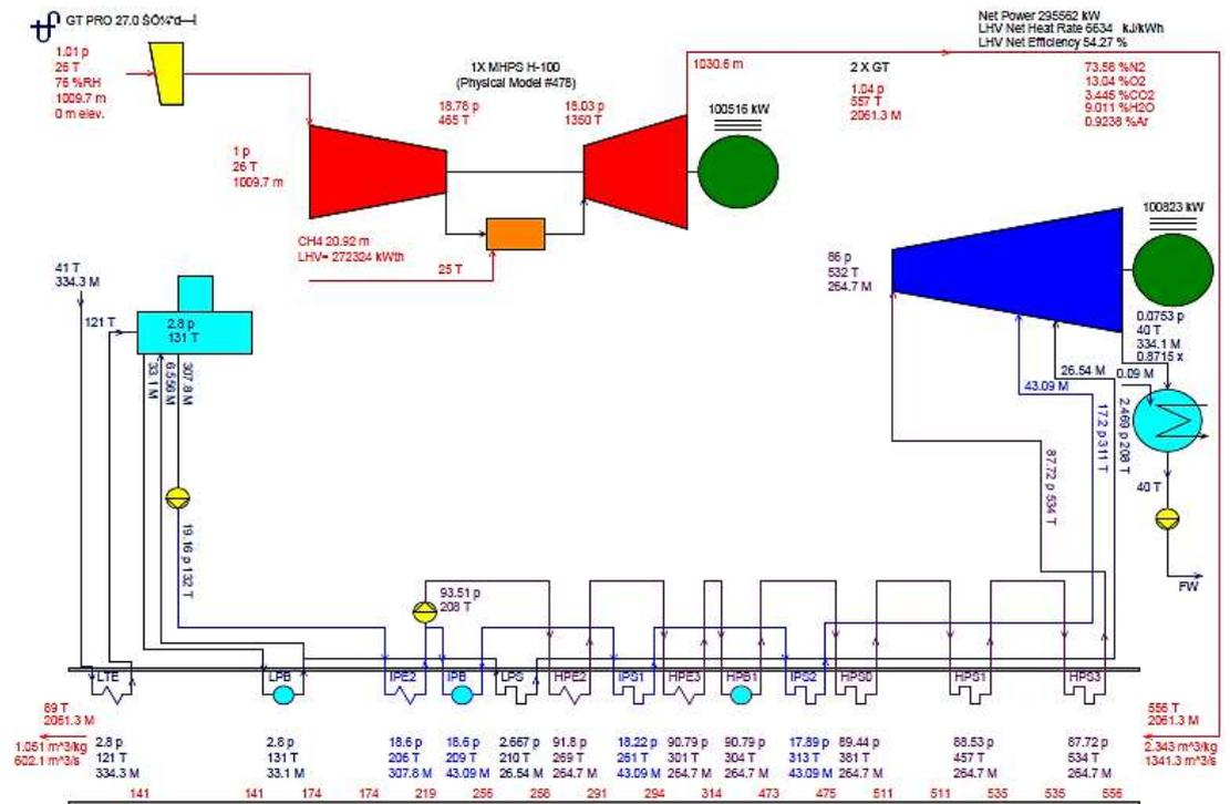
**Figure 2-7 Heat Balance Diagram of Heavy Duty GT**
