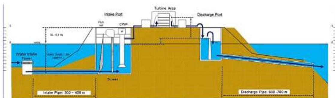
**Figure 2-15 Cross-section of Intake and Discharge Structures**
