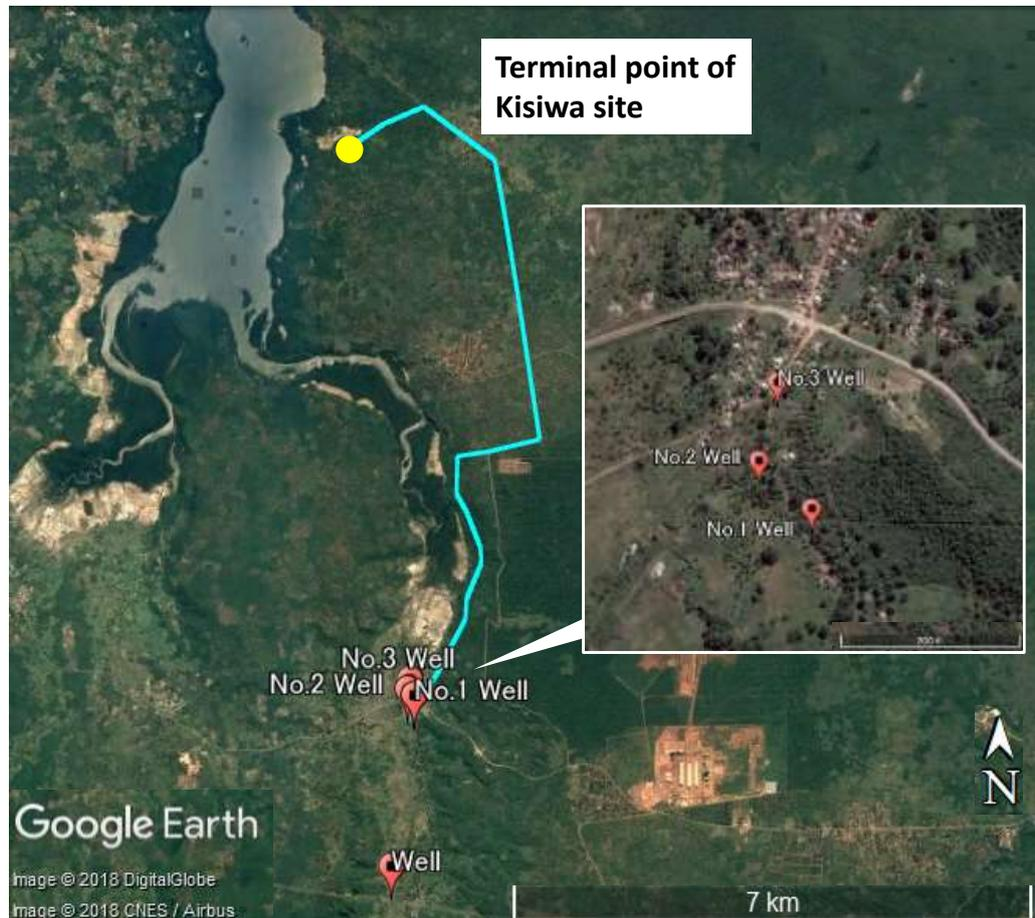
**Figure 2-33 Proposed Water Supply Pipeline Route**
