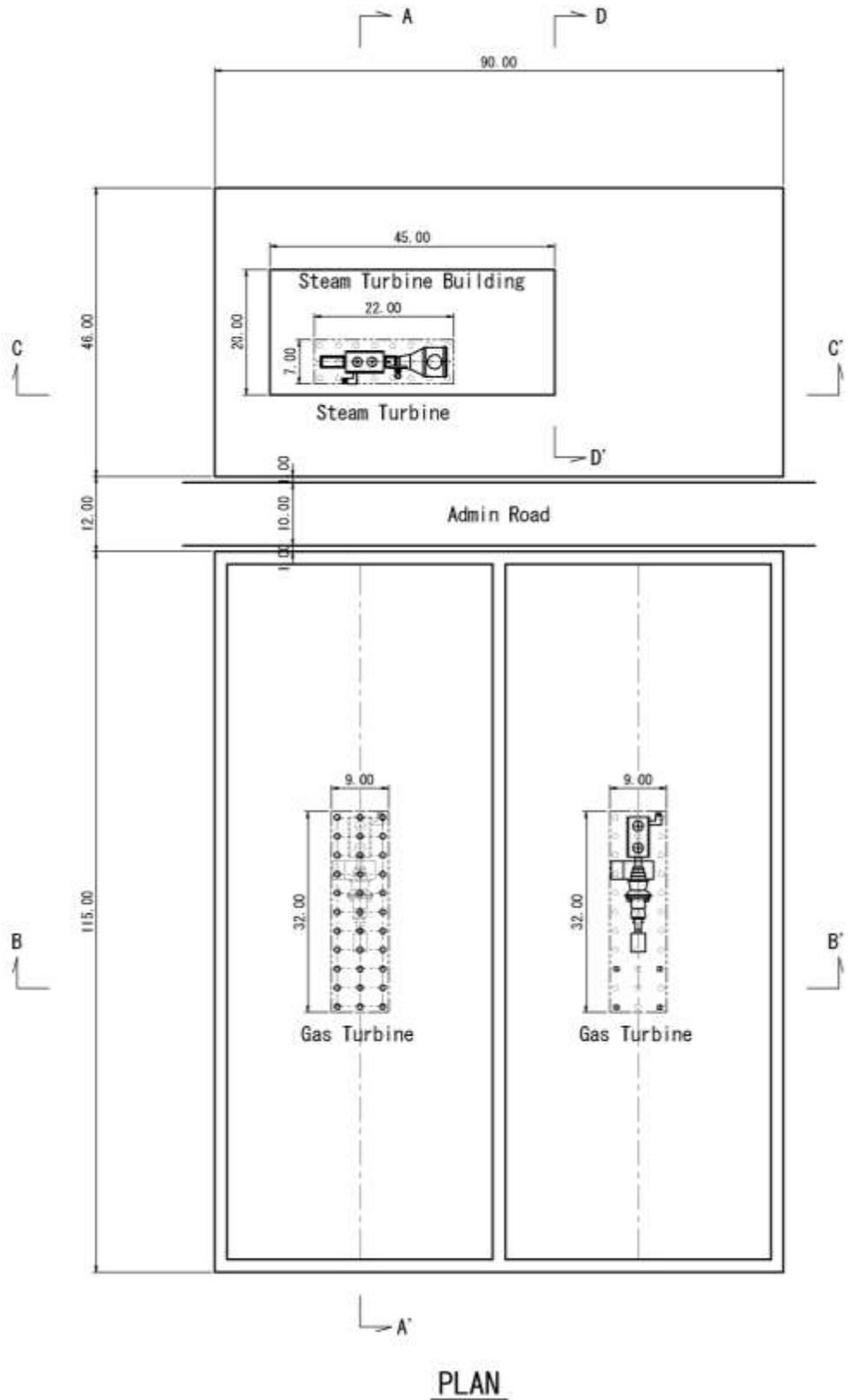
**Figure 2-26 Foundation Layout for GT and ST**
