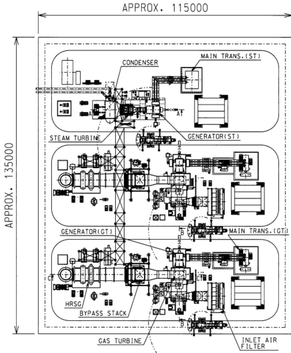
**Figure 2-6 Typical GTCC Layout of Heavy Duty GT with Seawater Cooling System**
