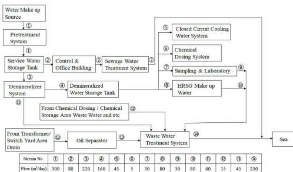
**Figure 2-14 Water Treatment Flow (Water Balance)**
