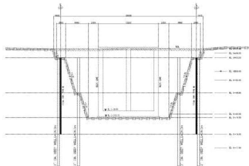
**Figure 2-29 Working Drawing of Water Intake/ Discharge Port (draft)**
