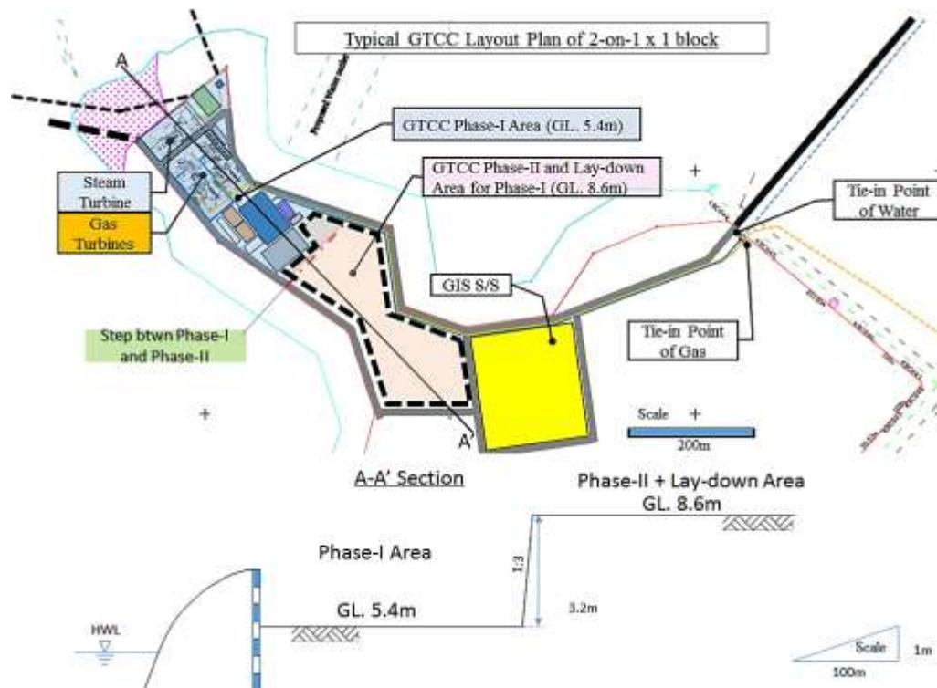
**Figure 2-30 Layout and Sectional View of Project Phase I and Phase II Areas**
