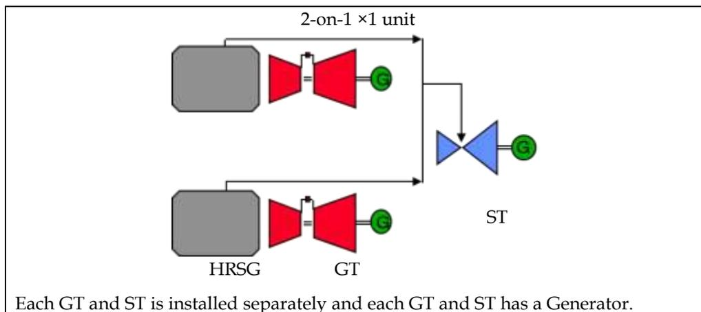
**Figure 2-8 Schematic Diagrams of multi-shaft 2-on-1 GTCC**
