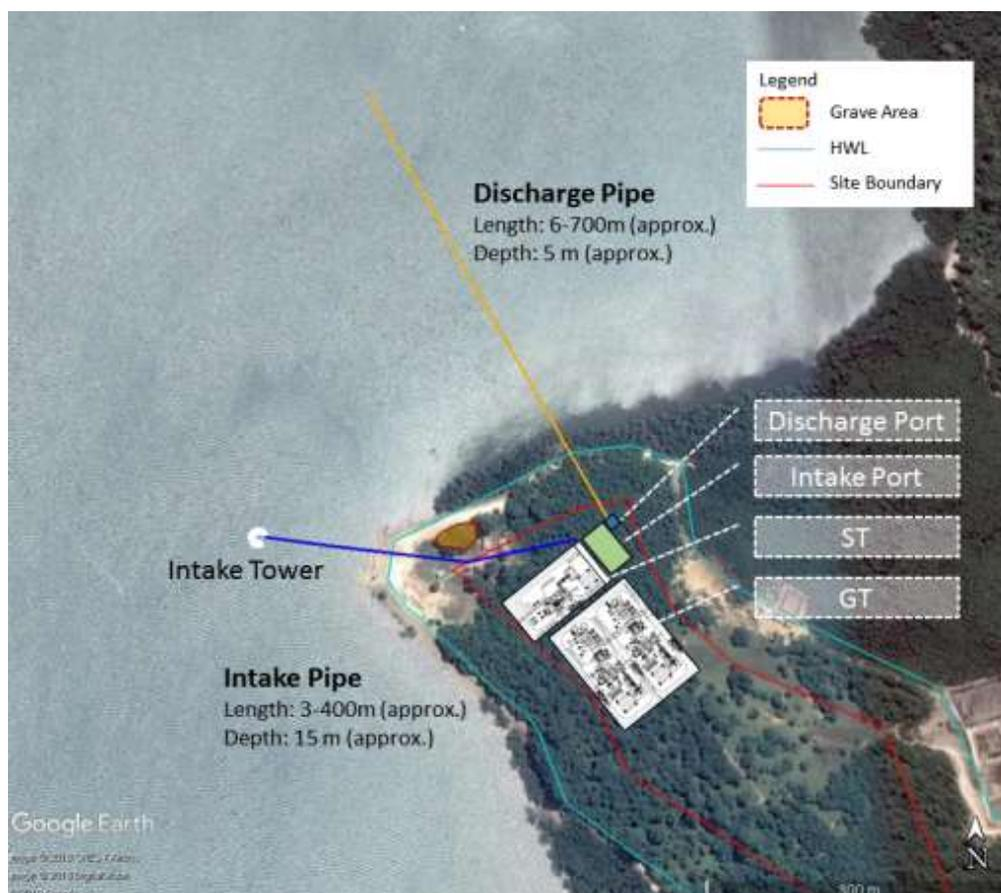
**Figure 2-16 Conceptual Layout of Intake and Discharge Streams**
