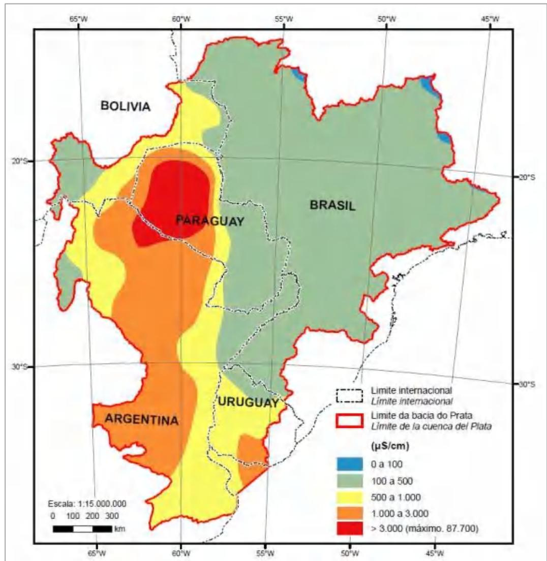
**Figure 48 – Groundwater salinity distribution. Source: Diniz *et al.* (2015)**
