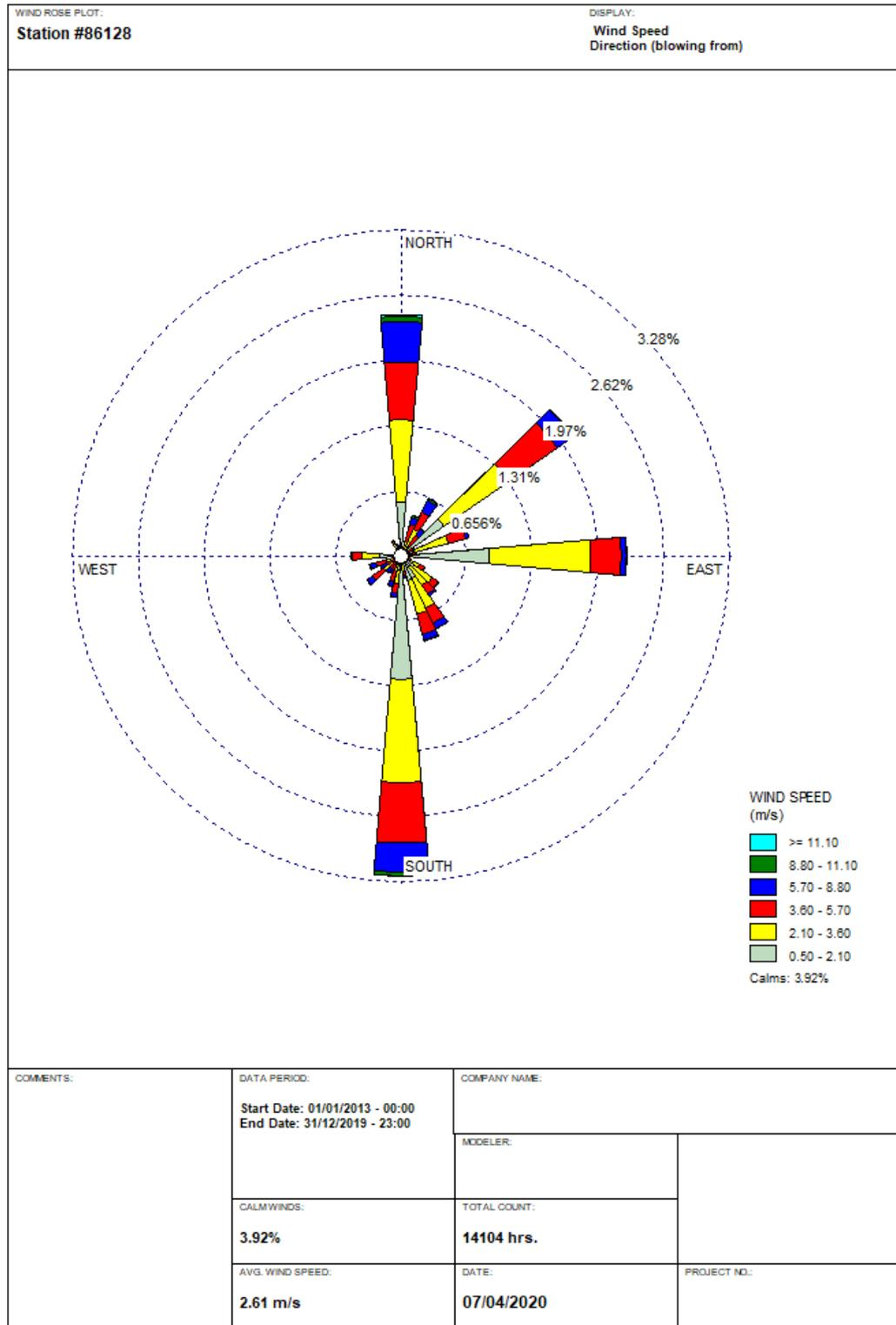
**Figure 22 – Wind rose observed at Pozo Colorado station**
