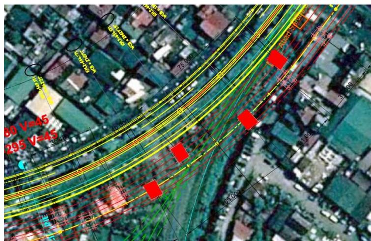
**Figure 4.2.59 Turnout tracks and existing track of PNR**
