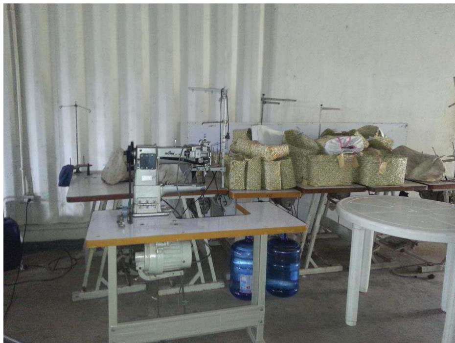
Figure 3.3 Heavy-duty Sewing Machine (used for sewing weaved bags and baskets)
