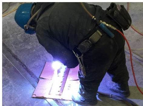
Figure 5.2.34 Thermal spray alloy Arc Plasma Spraying method
