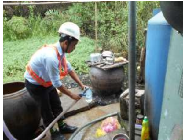
Sampling underground water
