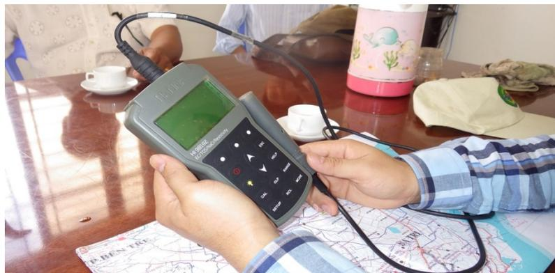
**Figure 2.3.12 Salinity Concentration Meter used at Son Doc 2 Sluice**
