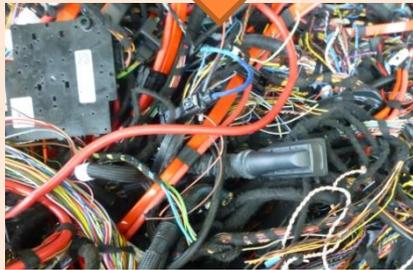
Wire Harness with socket and IC circuit can be processed with minute adjustment of crusher
