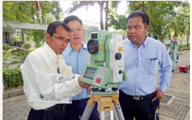
Demonstrating a crack measurement system (Kumonos Corporation)
