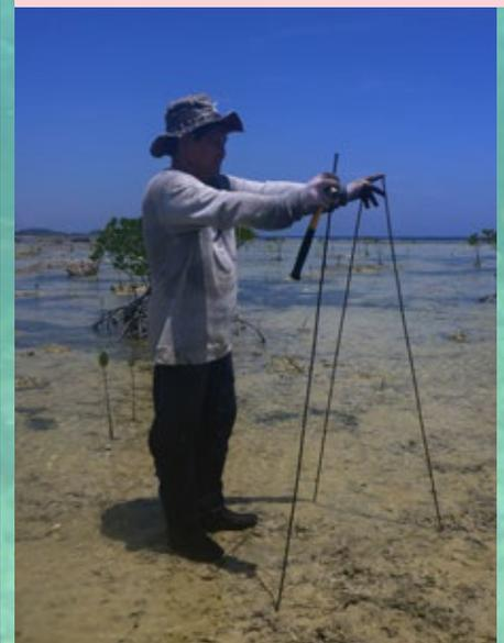
**Sediment depth determination using steel rod**
