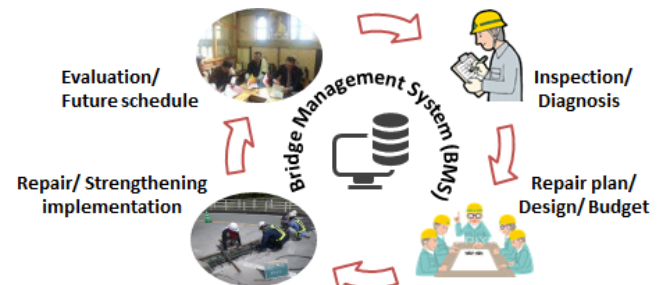
Figure2 Cycle of maintenance and BMS system
