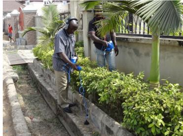
Microphone Leak Detector
