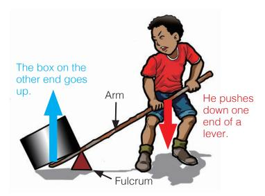
He is pushing down a lever to lift up a box.
