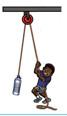
A <u>pulley</u> is a simple machine made up of a wheel through which a rope moves. A pulley helps us to lift an object.
