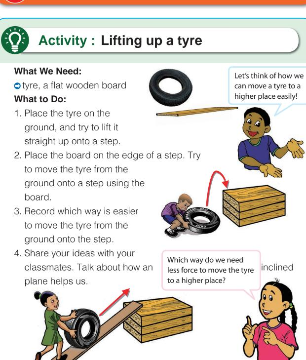
An inclined plane is a simple machine made up of a flat and slanted surface. An inclined plane can help move heavy objects easier from one level to another.
