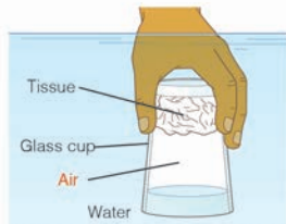
Air and water cannot occupy the same space at the same time.
