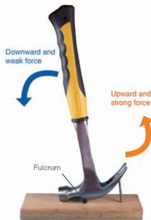
A lever changes the strength and the direction of a force.
